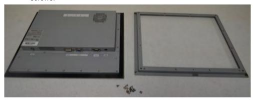
Now you should have the monitor, the rear metal bracket and the set of screws
