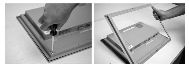
Once the monitor has been unpacked, lay it face down and unscrew the rear metal bracket by removing the silver M4 Phillips screws.
