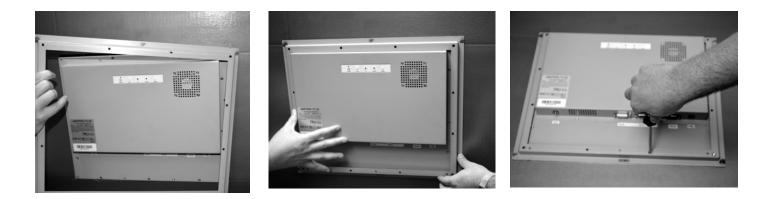
While holding the monitor in place, place the rear metal bracket in position and secure it with all screws. Ensure all screws are attached tightly.
