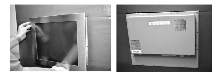
Next, slide monitor into the opening from the front. The back of the monitor will actually recess into the opening.
