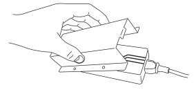
Attach the power supply to the mounting surface with 4 screws (not included).
