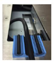
Plug cables into their respective connectors, then align the cables through the ports of rubber block. Be sure to keep black rubber cylinders in place for each unused port.
