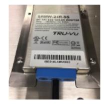
Tighten all 7 screws. The blue rubber block should not be able to move.
