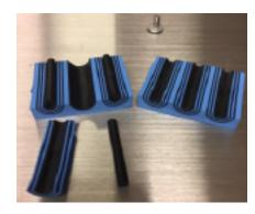
Open the blue rubber block. Remove inner black rubber cylinders for the ports needed for your cables. Peel back the necessary amount of layers in each port to ensure a tight fit for each cable. They must fit snugly.
