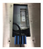
Remove the monitor's rear cover plate by removing all 7 screws.
