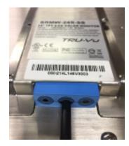
Then replace the rear cover plate. The blue rubber block should protrude slightly as shown.
