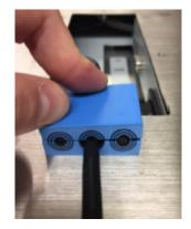
Replace the top half of blue rubber block. Position it at the bottom of the open stainless steel cover plate.
