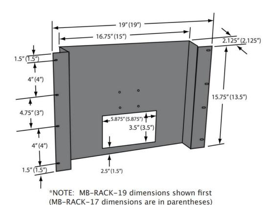
Why spend extra \$\$ for a rack mount monitor? Here is a low-cost, add-on solution to meet your flush mount needs. Just bolt the monitor adapter bracket onto the rear panel of your LCD monitor, and mount into any standard 19" rack. Although specifically designed for TRU-Vu 17" and 19" monitors, these mounts will fit most 17" & 19" displays, respectively. (Check that your display width will fit within the dimensions shown.)
